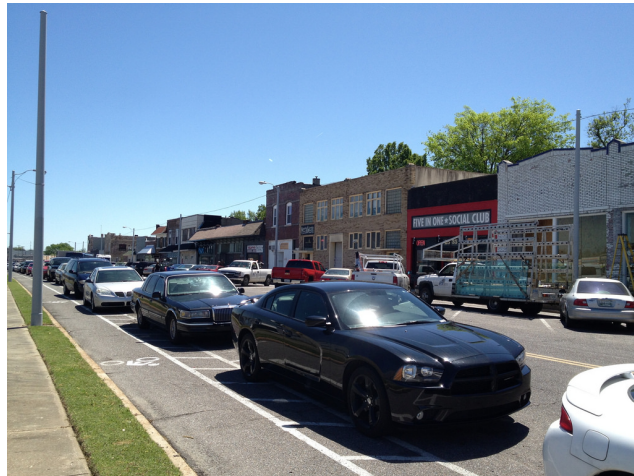
Figure 1: A parking lane protects the bicycle lane from vehicles in the travel lane. Image courtesy of USEPA .
