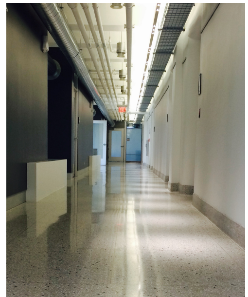
Figure 2: LED illuminated hallway, with diffused light to help mitigate glare of high gloss flooring. Image courtesy of IDEA Center
