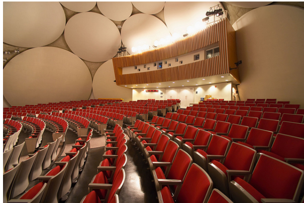
Figure 1: Auditorium of the Central Intelligence Building illustrating acoustic design features such as sound absorbent cloth seats, large plaster disks which enhance the acoustics of the space. Image courtesy of U.S. CIA Image Library
